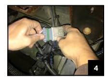
STEP 2: At rear of truck, locate and unplug the 7-way trailer harness plug
