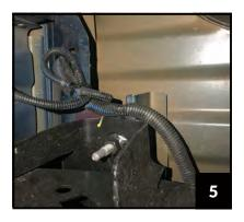
STEP 3: Attach modular wire harness to 7-way trailer port and re-attach plug from Step 2 to the second port on modular wire harness
